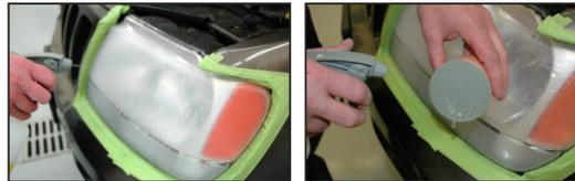
Using medium to high pressure, begin sanding to reduce the Green/Gray (P1000 grit) scratches to the Green/Gray (P3000 grit) scratches. **Add a mist of water to the surface if it becomes dry while sanding.** Make several passes on the surface of the lens. Avoid sharp edges or alignment pins on the lens to extend the life of the discs as this one disc will also be used for the other headlight lens. While sanding, a white residual or slurry on the lens indicates you are reducing the sand scratches.
