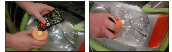
Using high pressure, rub the surface of the lens to remove the sanding scratches. When the orange pad becomes dry, continue by adding another quarter-sized amount of Rubbing Compound until the sand scratches have been removed and the lens is clear. **If additional clarity is needed or desired, add another quarter-size amount of rubbing compound and continue rubbing the headlight lens.**
