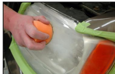
5. Wipe off the lens and inspect to ensure all the yellowing has been completely removed. If yellowing or portions of the surface layer still exist, continue sanding with Gold (P500 grit) discs until they are completely removed.
