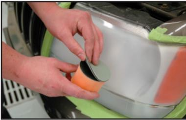
10. Using a spray bottle, apply enough water to dampen the Green/Gray (P1000 grit) foam sanding disc and the lens surface before sanding.
