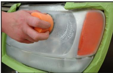
**Tip:** Extra sanding on this step will make the next step easier and improve the final clarity of the headlight lens.
